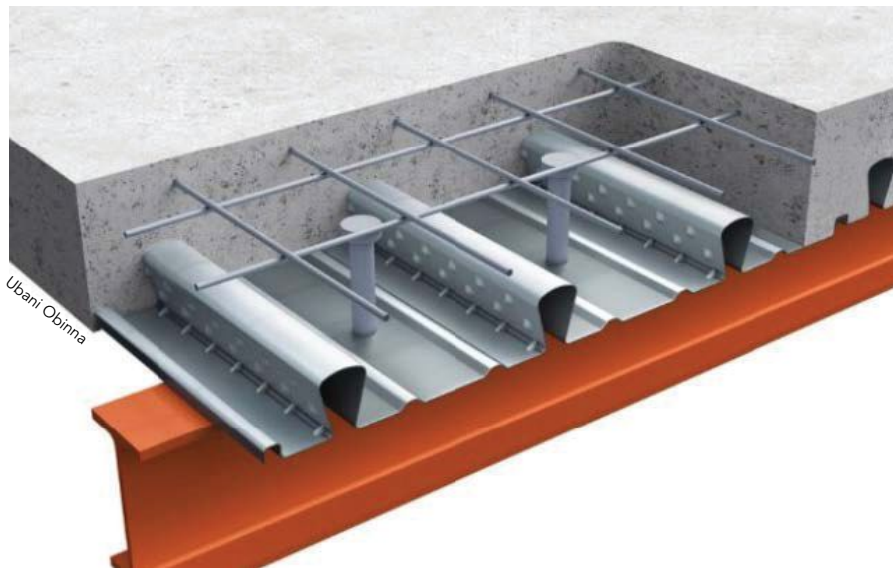
Fig. 1. Schematics of a composite steel floor slab.
